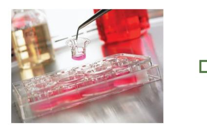
Transwell filter insert (0.4 µm pore size)
