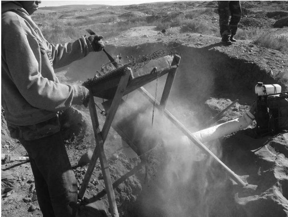
Figure 2. Sifting alluvial soil using gravitation and compressor. Zaamar, June 2013. Photo by G. Munkherdene. A color version of this figure is available online.
