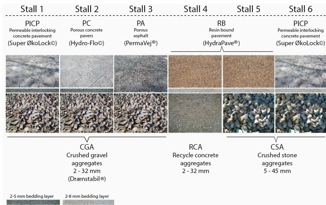
Figure 2. Diagram showing the combination of surface layer, bedding layer and sub-base layer of PP systems tested in six stalls, including photos of individual layer materials, where CGA = crushed gravel aggregates; RCA = recycled concrete aggregates; and CSA = crushed stone aggregates.
