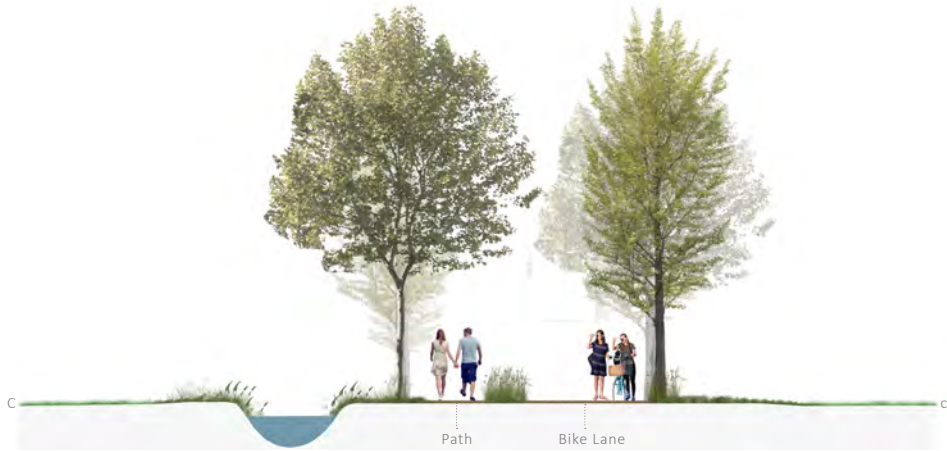
Section C-c Allées are planted across the portions of the trail that are not directly situated in the wet meadows. The species are primarily native and their selection is based on the trail surroundings. In drier areas, like the middle of the fjord by the canal, species like European aspen ( Populus tremula ) are chosen, while by Engfjorden, more wet-tolerant species, like white willow ( Salix alba ), are planted instead. The allées will help create smaller ecological corridors and will compliment the existing allée cultural landscape features that already exists along some of the roads in the fjord.
