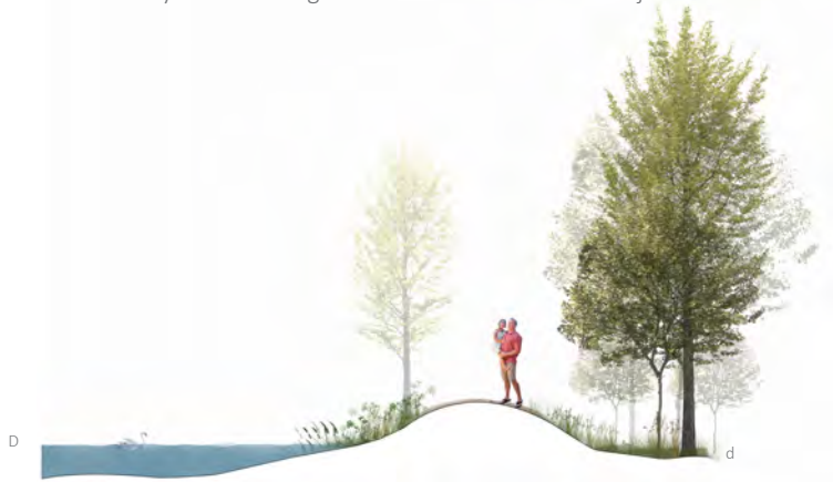
Section D-d The topography is raised by 1 metre to create a berm at the border between Engfjorden and existing agricultural fields to ensure that they will not get flooded as portions are situated within the lowest contours in Sidinge Fjord. This will ensure that a diversity of landscape types can co exist in area.
