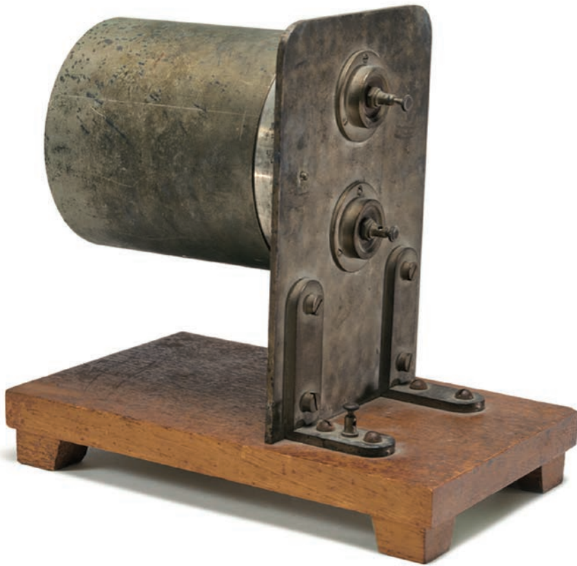
9. Ionization chamber used by Marie and Pierre Curie. Photo by Gabriel Hildebrand, Nobel Museum.
