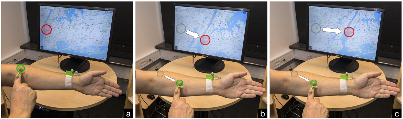
Figure 6. a) Scrolling the map to center New York by swiping horizontally on the arm. b) 1-to-1 mapping results to a downward drift on vertical direction on the display, and a transition too short on horizontal direction. c) using the models allows to map touch to the content on a display as users intended to.
