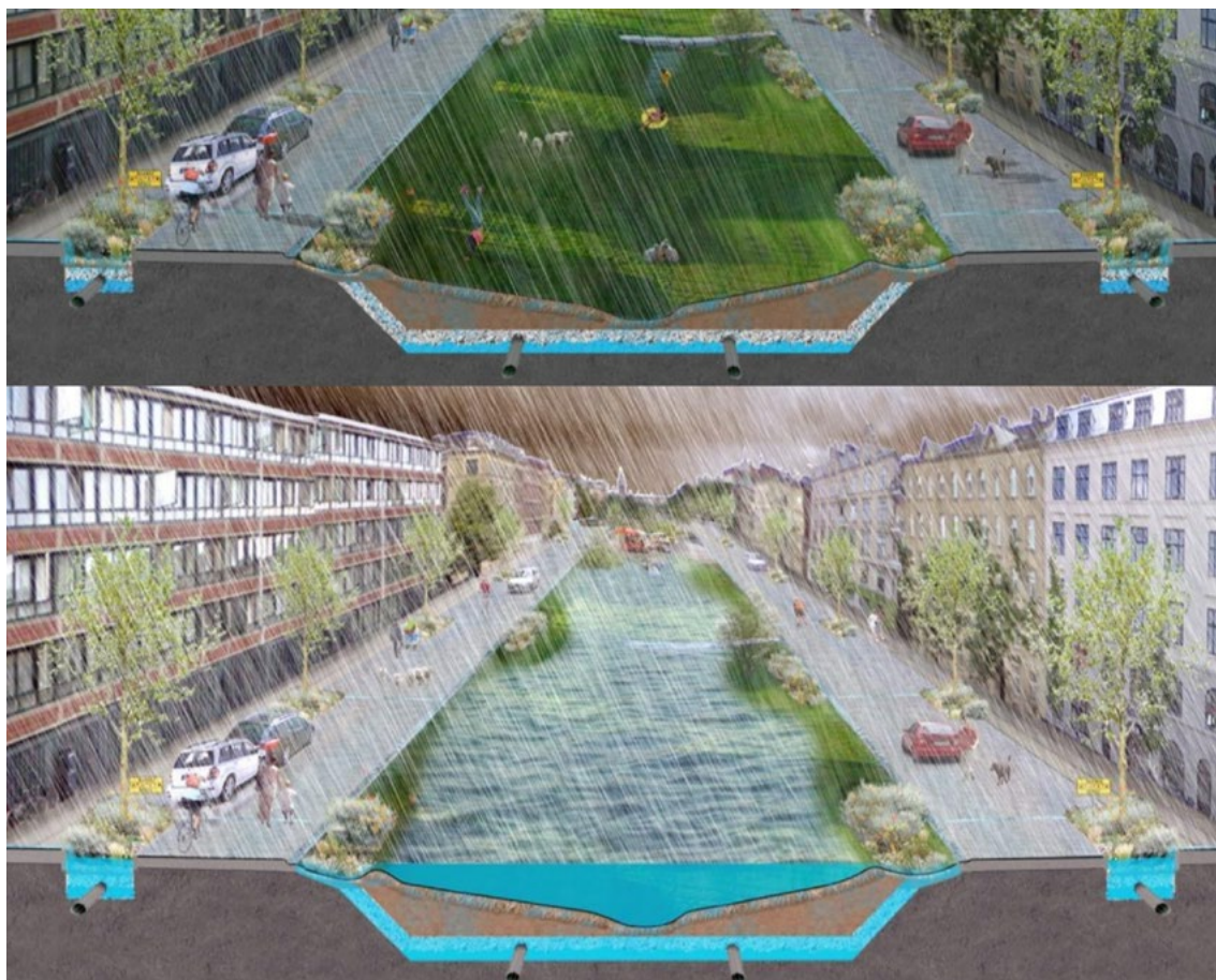
Figure 14 – Concept design for Copenhagen detention road (top image) which is designed to become an open water body during intense rain (bottom image) (source: City of Copenhagen)
