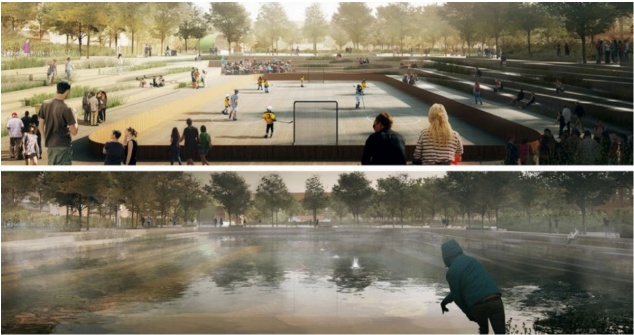
Figure 15 – Concept design for detention area in Enghaveparken park in Copenhagen (top image) that turns into open water body during intense rainfall (bottom image) - (source: http://citiscopes.org/story/2016/why-copenhagen-building-parks-can-turn-ponds )
