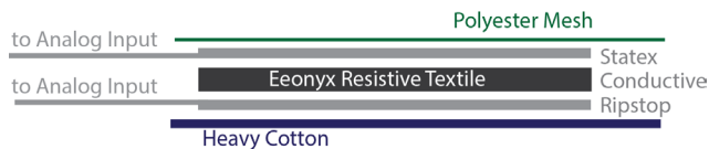
Figure 5 – Cross Section of zPatch
