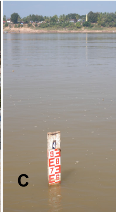
Figure 3. A. Water level at Chiang Khan for selected years. The average value is based on data from 1980 to 2013. Redrawn from the Mekong River Commission (2017); B. Water level scales by Chiang Khan on 1 January 2010 measured in relation to the zero gauge at Chiang Khan town (194 m above MSL); C. The water level of 3.6 m as shown in B.
