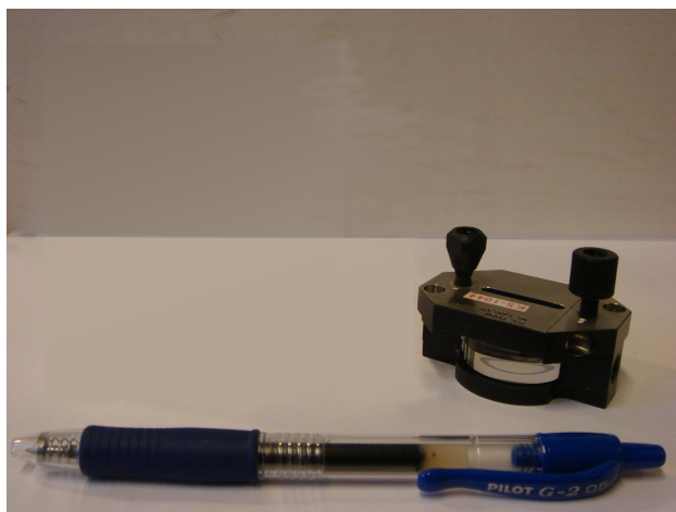
Figure 5.1: A light scattering flow cell from Wyatt Technology. Other companies use flow cells of other designs.
