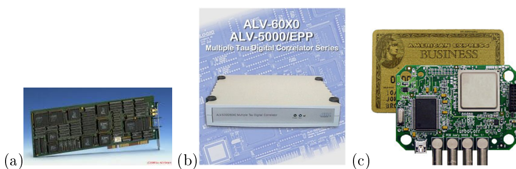
Figure 4.2: Three different digital autocorrelators from companies ALV Brookhaven Instruments: (a) ALV 5000, (b) ALV 5000/EPP, (c) TurboCorr
