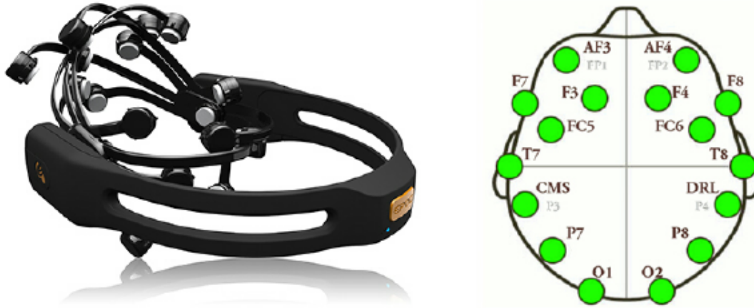
Figure 7.3: A picture of the Emotiv headset as well as the positions of its 16 electrodes. Taken from https://www.researchgate.net/profile/Nicola_Catenacci_Volpi/publication/284031383/figure/fig1/AS:296815892156418@1447777831163/fig-1-The-Emotiv-EPOC-and-the-electrodes-location.png .
