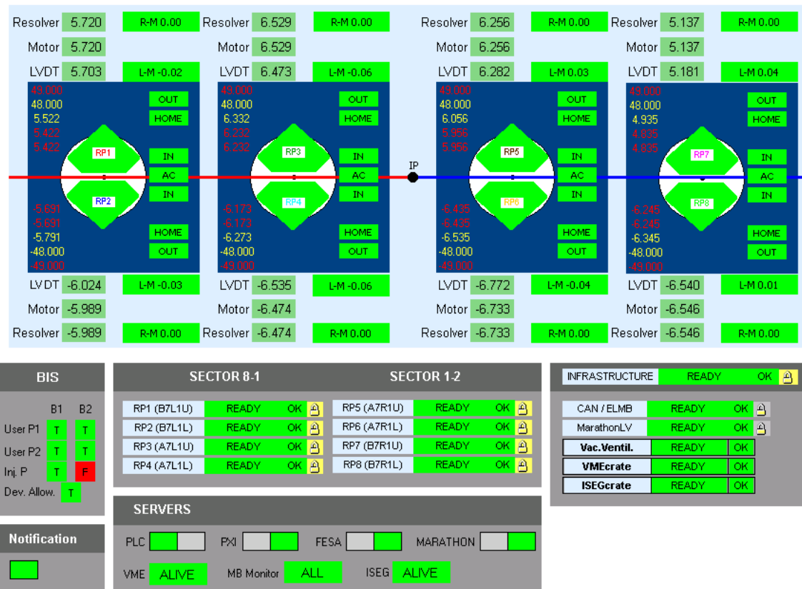
Figure 18. A cutout of the ALFA DCS top panel with the RP positions retrieved from the LVDTs, the motor steps and the resolvers. The lower part indicates the status of the Beam Interlock System (BIS), the power status of all detectors in sectors 8–1 and 1–2, the status of the infrastructure components and of all servers. The snapshot is from the \beta^* \approx 90 m run in October 2015 with RP positions at 10\sigma of the beam envelope.
