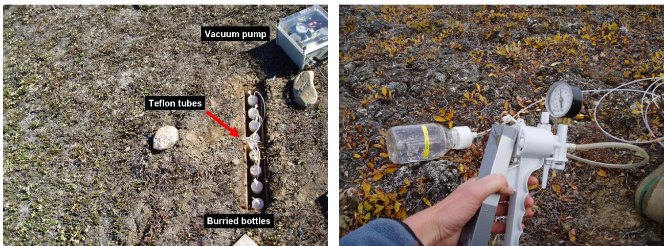
Fig 9.13 Collecting bottles at the K3 site. Bottles are hidden in the wooden box. To apply vacuum use the automatic pump (mid) or the hand pump (left)
