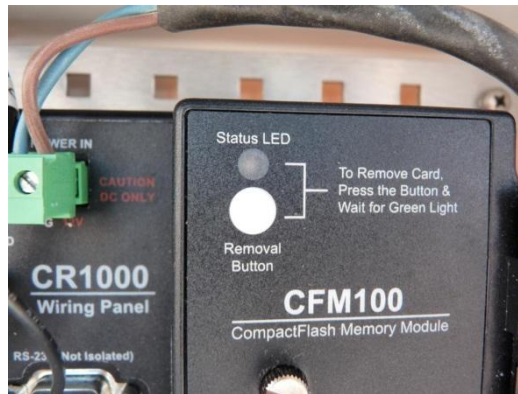
Fig 2.8 CFM100 CompactFlash Memory Module with turned off diode that indicates the CF card is ok (as on picture). If the Status LED is orange then the CF card is NOT working.
