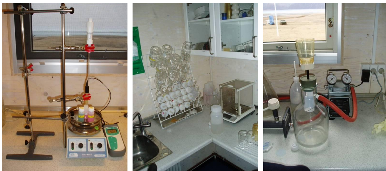
Fig 8.1 Laboratory in Zackenberg. pH meter next to the magnetic stirrer. The pH electrode is held by the lower clamp and the acid dispenser is held by the upper clamp (left). Analytical balance (middle). Device for filtration of water samples. Filtered water is collected directly into a clean sample bottle. Vacuum is applied by the electrical pump connected to the glass bottle (right).
