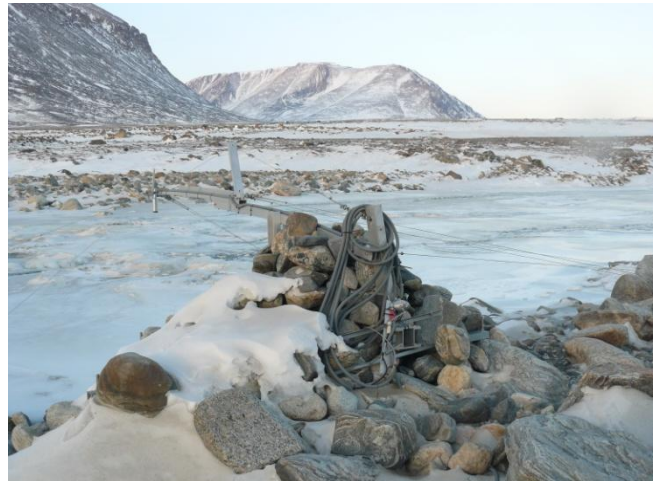
Fig 7.9 Old storage of cable and sensors during winter
