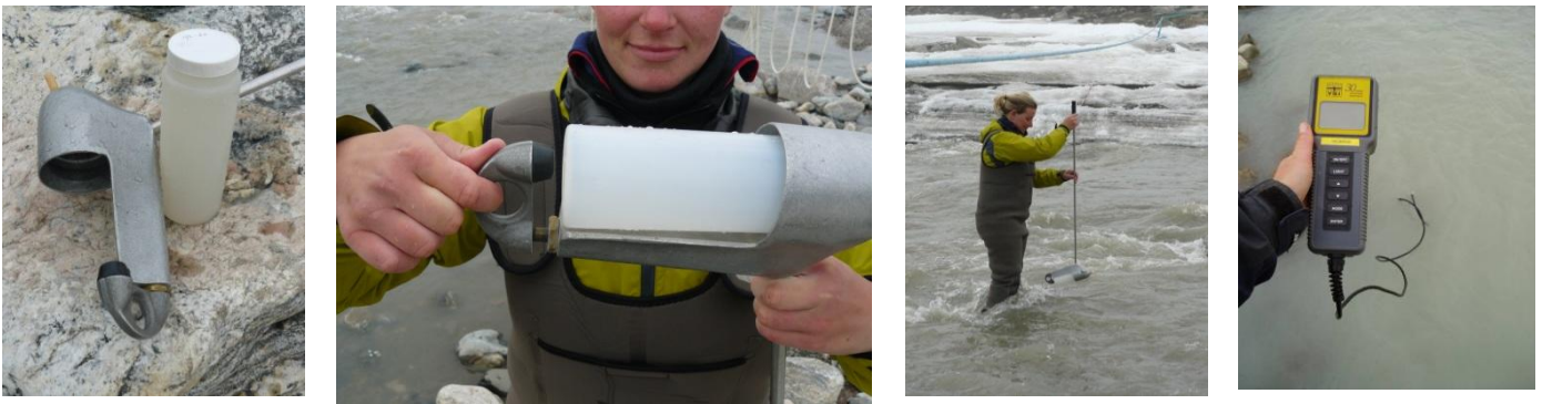
Fig 7.15 Depth integrating sampler and conductivity meter used at the daily sampling.
