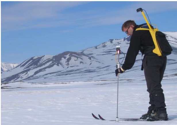
Fig 2.10 Magnaprobe in use. The metal probe is pushed into the snow and down to the ground surface. The floating basket moves up and down and gives the position of the snow surface. The probe is connected to a CR10 datalogger. A depth reading and a GPS position are made when you press the thumb switch on the handle.
