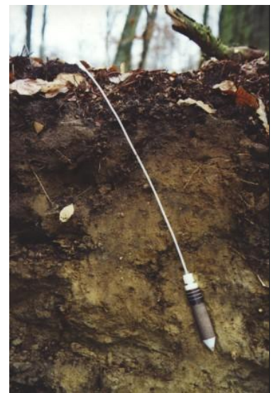
Fig 9.10 Installed suction probe. A teflon tube connect the probe to the soil surface. Photo not from Zackenberg.
