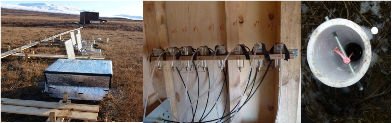
Fig 10.18 Chamber 2 covered with box for dark chamber measurements (left). Water traps inside the hut (mid). Looking into white tube with diver (right).
