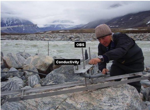
Fig 7.8 Metal frame for installation of OBS, diver and Conductivity sensor
