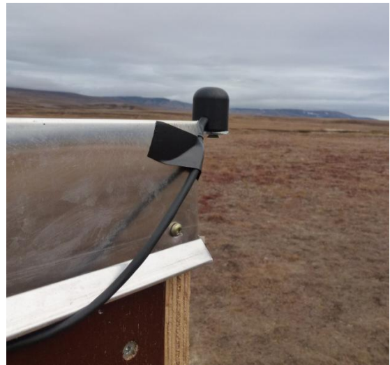
Fig. 10.20 Par sensor mounted on the south-western corner of the hut.
