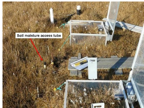
Fig 10.19 Looking down into the area in front of the chambers. Between the chambers there are fixed metal probes, use the top of these to measure the active layer (left). There are three soil moisture tubes between chamber 1-2, 3-4 and 5-6.
