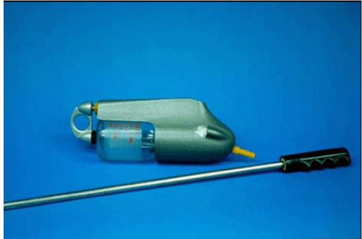
Fig 7.14 US DH-48 depth integrating sampler with 500 ml plastic bottles. To remove or insert the bottle; pull back and turn the handle in the back
