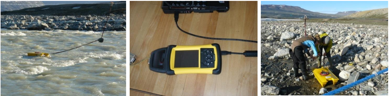
Fig 7.13 Q-liner boat in the river (left). PDA connected to computer (mid). Attaching the Q-liner to the wire (right)
