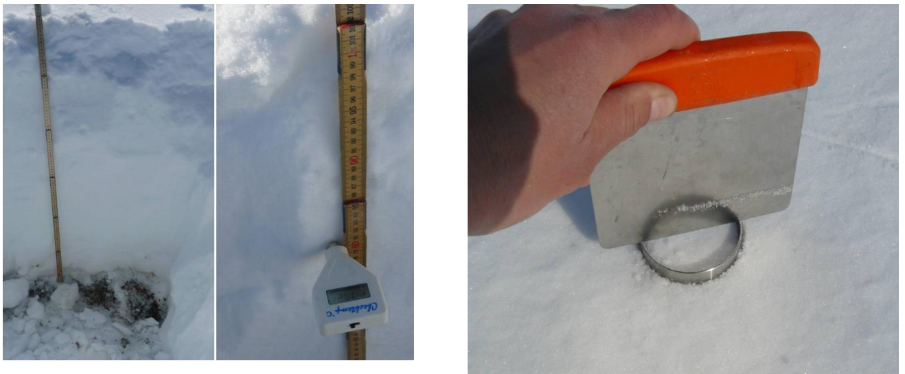
Fig 2.15 Snow pit without basal ice. Temperature recordings. A small ring (100 cm 3 ) is used to sample the surface snow.
