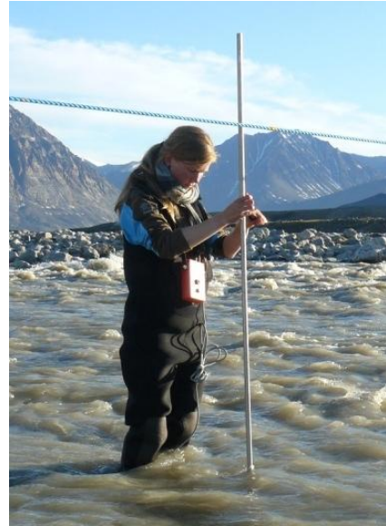
Fig 7.12 Standard velocity profile in the river and an example of measuring velocity at two different water depths.
