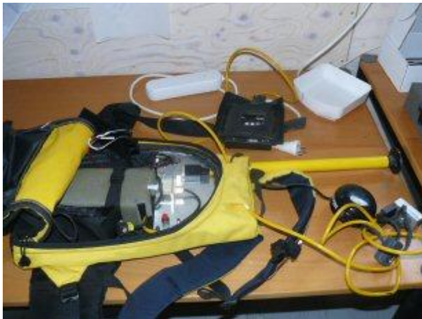
Fig 2.12 The data logger in the bag pack with GPS antenna, cable and switch to mount on the probe.
