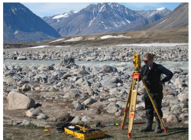
Fig 12.7 Total station at the river bank and equipment used
