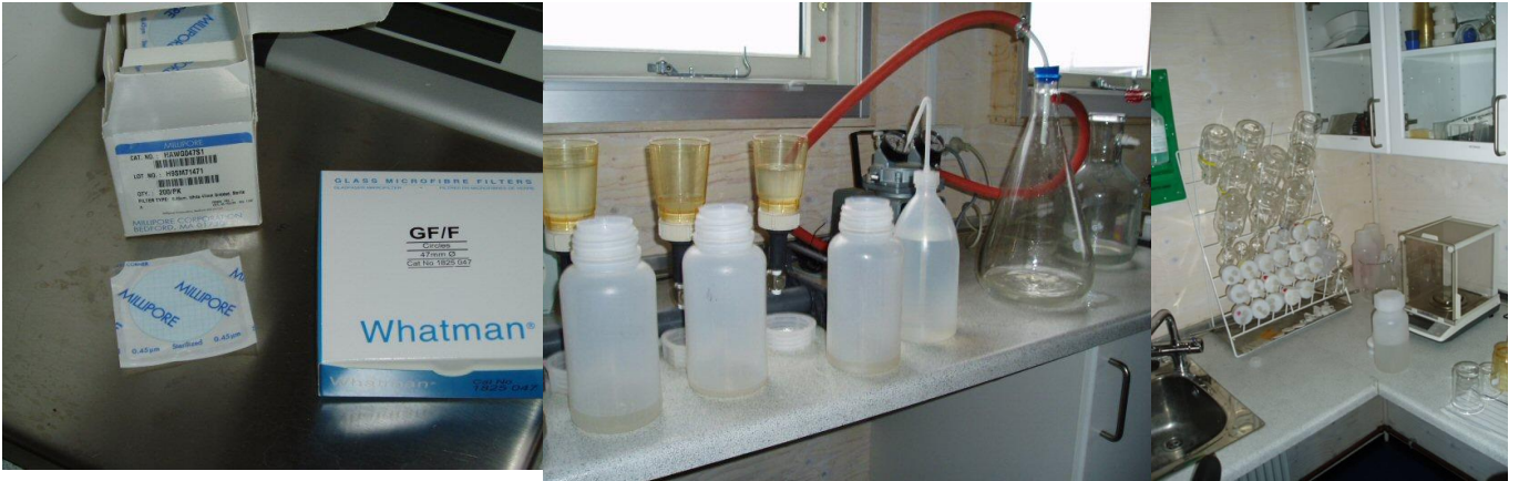
Fig 8.2 Whatman GF/F filters are used for filtration of suspended sediment samples (left). Milipore filter assembly connected to the vacuum pump. Three samples can be filtered at the same time (Mid). Analytical balance (right).
