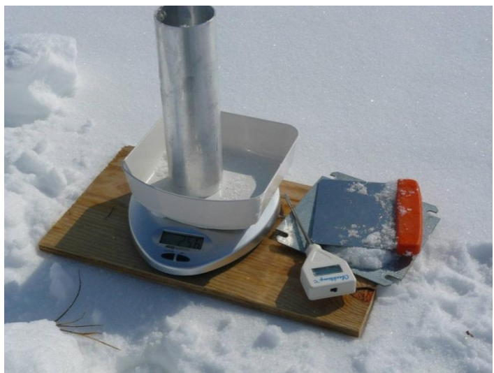
Fig 2.14 Equipment used for sampling in the snow pit.
