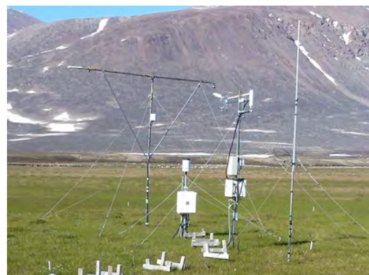
Figure 9: MM2 with energy balance mast, behind precipitation gauge and eddy covariance tower.
