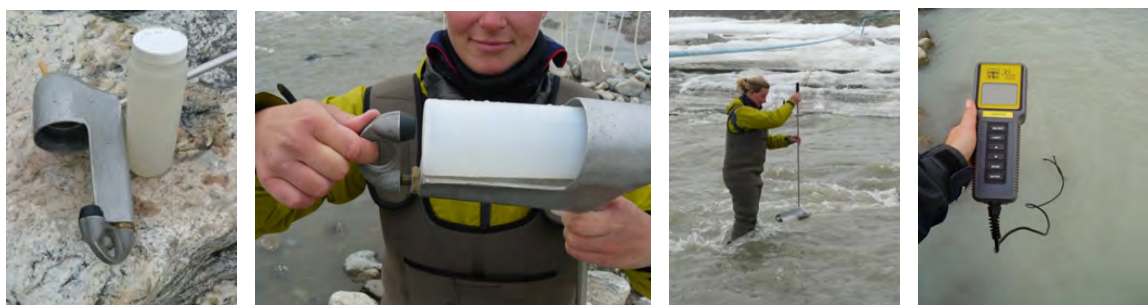
Figure 49: Depth integrating sampler and conductivity meter used during morning and evening sampling.
