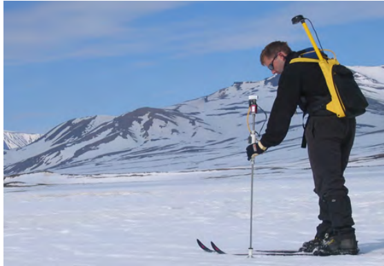
Figure 15: Magnaprobe in use. The metal probe is pushed into the snow and down to the ground surface. The floating basket moves up and down and gives the position of the snow surface. The probe is connected to a CR10 datalogger. A depth reading and a GPS position are made when you press the thumb switch on the handle.
