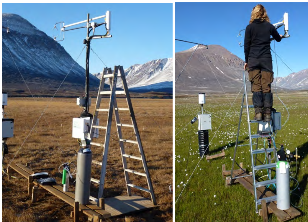
Figure 66: Setup for span testing or calibrating Licor7200. Left; the ladder is used for connecting or disconnecting the Bev-a-line tube for the air intake on the mast (where the white tube is connected to the licor house), Nitrogen and span gas, the computer is connected to the Licor7200 underneath the white enclosure using a RS232 cable. Right; calibration ‘in action’ the reference gas is connected to the licor7200 through the bev-a-line tube and in situ measurements are read from the PDA and noted in the calibration sheet.
