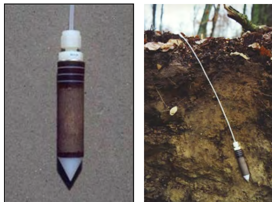
Figure 55: Left: Suction probe used in Zackenberg. Pore size: 2 microns. Right: Installed suction probe. A teflon tube connect the probe to the soil surface. Photo not from Zackenberg.
