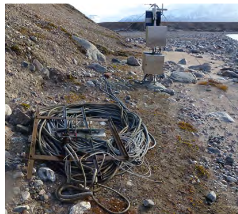
Figure 44: Storage of cable and sensors during winter, by the old hydrometric station
