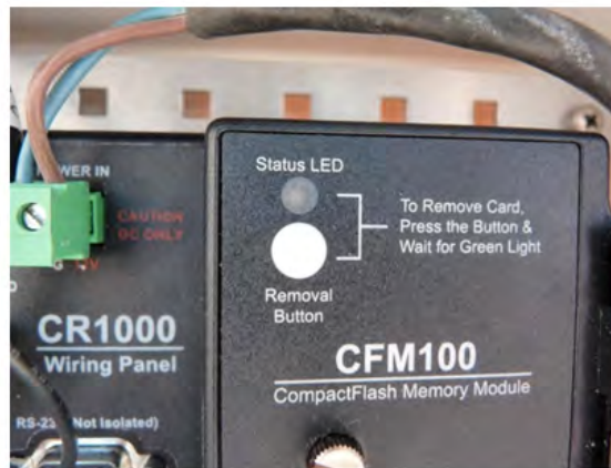
Figure 10: CFM100 Compact Flash Memory Module with diode turned off that indicates the CF card is ok (as on picture). If the Status LED is orange then the CF card is NOT working.
