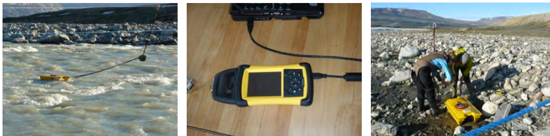
Figure 46: Q-liner boat in the river (left). PDA connected to computer (mid). Attaching the Qliner to the wire (right).
