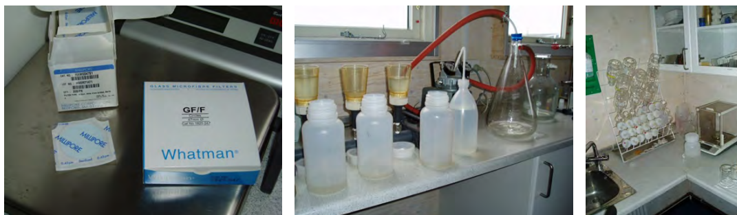
Figure 51: Whatman GF/F filters are used for filtration of suspended sediment samples (left). Milipore filter assembly connected to the vacuum pump. Three samples can be filtered at the same time (Mid). Analytical balance (right).
