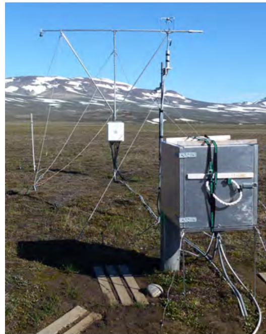
Figure 8: MM1 with energy balance mast, behind eddy covariance tower and enclosure instruments.
