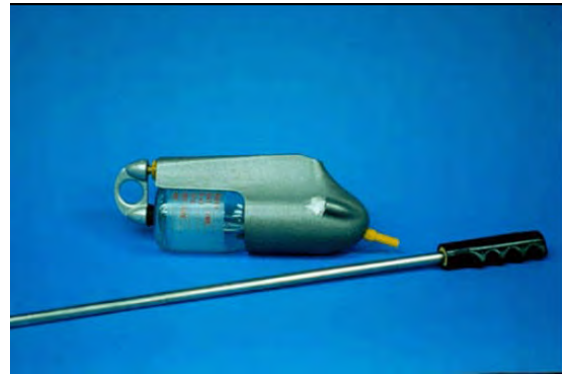
Figure 48: US DH-48 depth integrating sampler with 500 ml plastic bottles. To remove or insert the bottle; pull back and turn the handle in the back.
