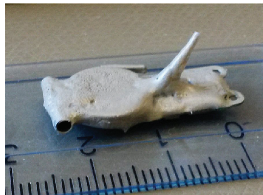
Figure 1. The activity data logger ready to be mounted on a bird. Most of the mass and volume is the button-cell battery (flat circular 10 mm structure to the left). The upward-pointing structure is the 'light-stalk', an acrylic tube that conducts ambient light down to a light sensor mounted inside the logger.
