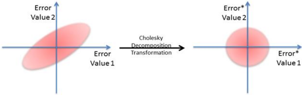
Figure 5: Hypothetical 2-dimensional example of the forecast error unification via Cholesky decomposition. Before transformation, the DLM forecast errors are mutually dependent, as illustrated by the tilted ellipsis. The Cholesky decomposition of the forecast variance matrix is found, and this is used to transform the forecast error vector. The values in the transformed forecast error vector are now mutually independent and will each follow a standard normal distribution, as illustrated by the circle. The transformed forecast error vector can be thought of as a point within this circle, and the distance between (0,0) and this point is taken as the unified forecast error.
