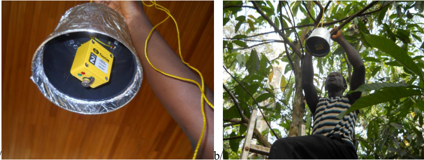
Figure 5a and b show a Tinytag in an aluminium foiled pot and a farmer mounting the pot in the cocoa canopy
