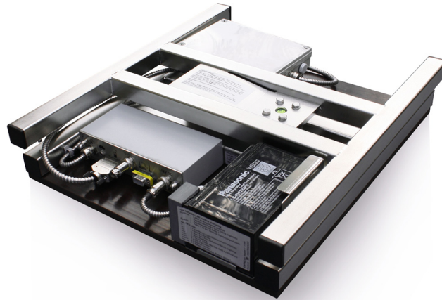
Fig 1. The Capaz scale before installation. The Capaz hivescale is an H-shaped platform made from aluminium and stainless steel, with the dimensions 420 x 480 x 86 mm (long x wide x high). Data are transmitted by cell phone. The rechargeable battery (12 V) lasts for 200 days. Ambient temperature and humidity are measured by default. Additional equipment is the rain collector and brood temperature sensor. Changes of the standard setup of the scale are done via the computer software. Photo: Capaz.
