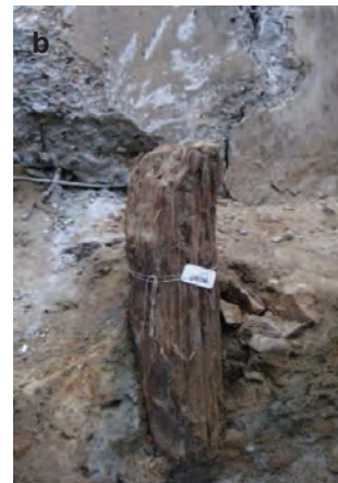
Figure 4.2: a) The excavation site at Kongens Nytorv showing the waterlogged nature of the moat just before retrieval of the poles. The bucket contained a pump that ran constantly to lower the ground water level. Picture © Museum of Copenhagen. b) Pole situated outside the moat close to a concrete cable station placed under ground in modern times. The pole was clearly in a bad condition compared to the poles within the moat and is most likely attacked by brown rot fungi due to aeration of the site.
