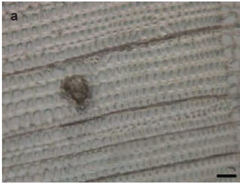
Figure 5.1 a: Cross section of Norway spruce ( Picea abies ) latewood reference material viewed in light microscope. Scale bar = 50 \mu m.
