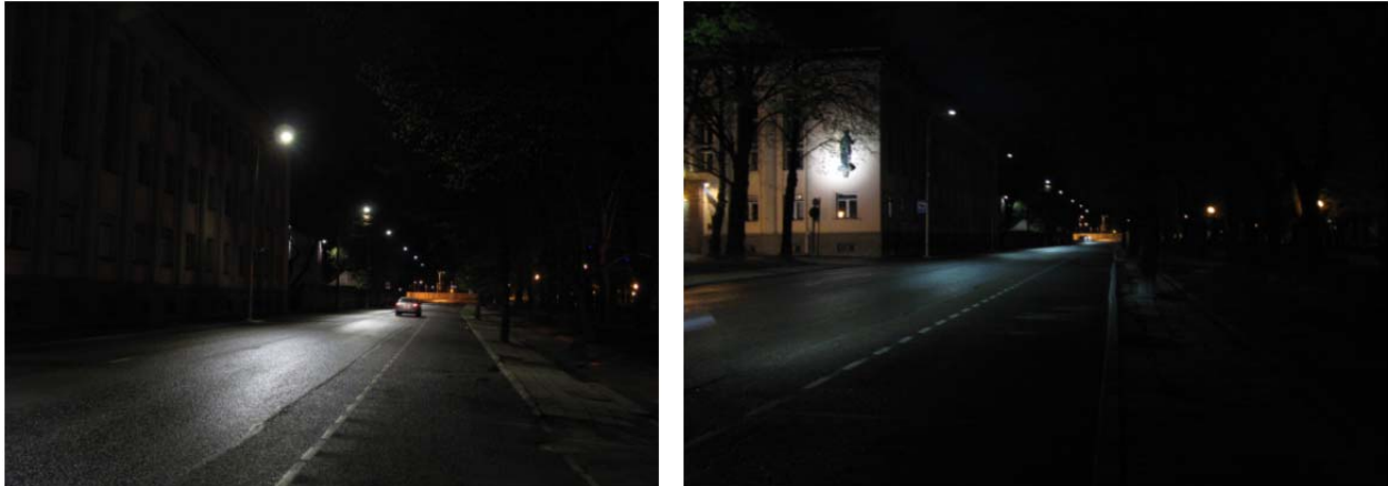
Figure 44: Dimming in Vabaduse Alley, 107 W LED 100% (left) vs. 107W LED 20% (right)
