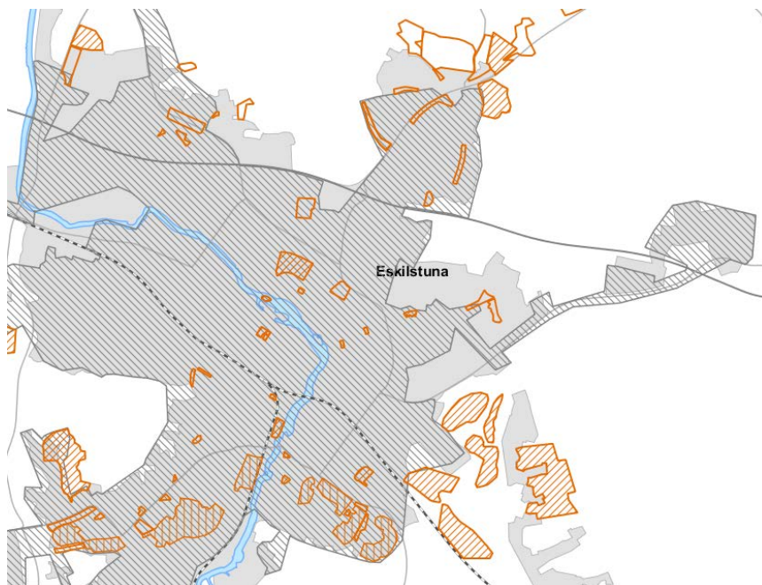
Figure 31. District heating and housing. After deregulation of the planning system, it is no longer possible to assign districts for district heating. The map shows the urban areas currently provided with district heating (grey hatched) and areas planned for housing by the Eskilstuna Comprehensive plan 2013/2030 (brown hatched). No information is available regarding the future energy supply of the assigned housing areas outside the district heating areas. With the deregulation of the municipal planning monopoly, the future heating in these districts will be decided by agreements between the developer and the Eskilstuna Energy & Environment enterprise. Whether district heating will be an option for the developer depends on decisions made by Eskilstuna Energy & Environment as to the profitability of including new districts in the heating system.
