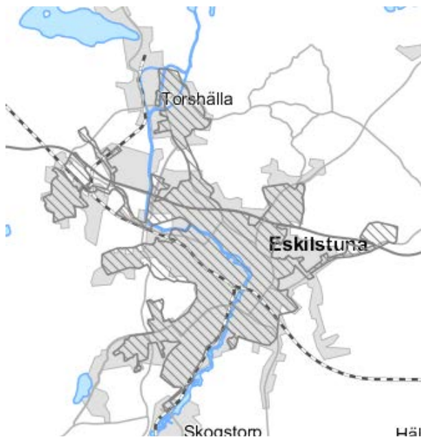
Figure 28. Distribution network for district heating
