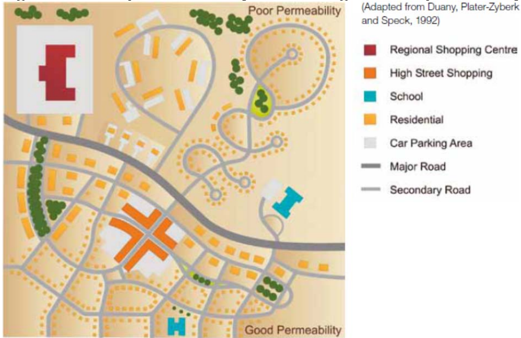
Figure 4.4. Examples of street layouts with high and low permeability
