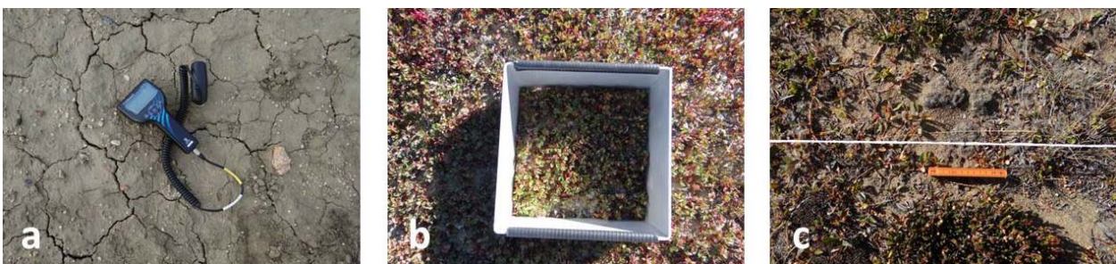
Figure 6.24 a) HS2 Hydrosense soil moisture measurement tool. b) Exemplary plot for biomass sampling, c) Land cover photograph. Photo: Jennifer Sobiech-Wolf.
