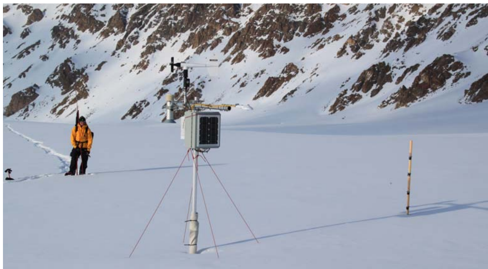
Figure 6.1 The automatic weather station (AWS, 860 m a.s.l.) on Freya Glacier during the spring survey (5 May 2013, snow height ~70 cm) and at the end of summer (14 August 2013) after an ice loss of 80 cm. Photos: Geo Boffi and Bernhard Hynek.
