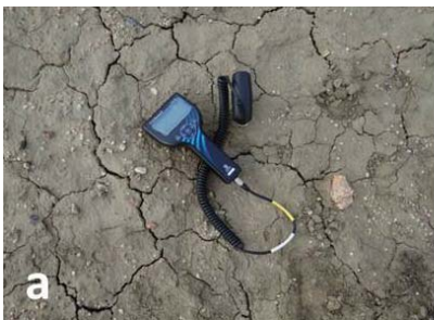
Figure 6.24 a) HS2 Hydrosense soil moisture measurement tool. b) Exemplary plot for biomass sampling, c) Land cover photograph. Photo: Jennifer Sobiech-Wolf.
