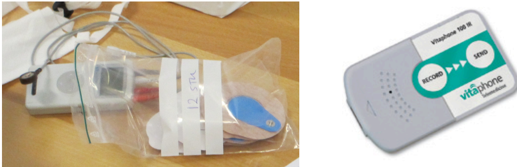
Figure 1. Left, a Holter-monitor with extra patches ready to be handed over to a patient. Right, an event card (Copyright by http://cardiologyforless.com/image.php?type=P&id=1541 ).
