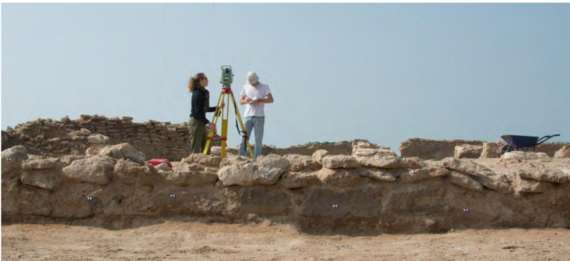
Figure 7.11: Measuring photo targets on wall elevations.
