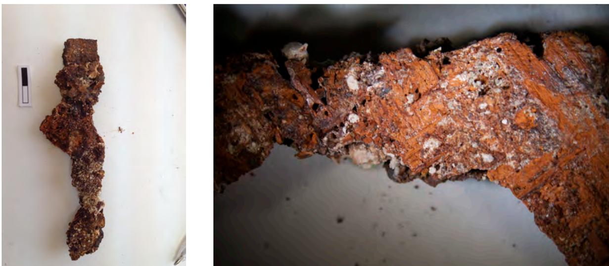
Figure 15.5: An untreated iron knife with a thick corrosion layer. Attached to the surface are residues of organic material. (UG & OF-3914)
