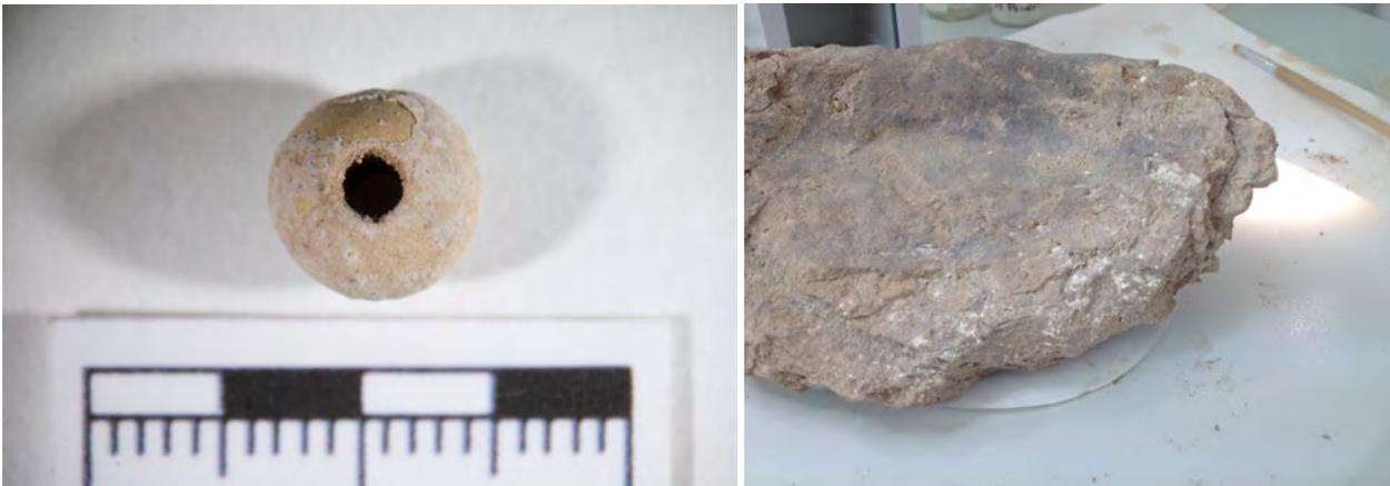
Figure 15.1: An example of visual efflorescence of salt on the exterior of a ceramic bead and a low fired ceramic fragment. (OF-3731 & UG)
