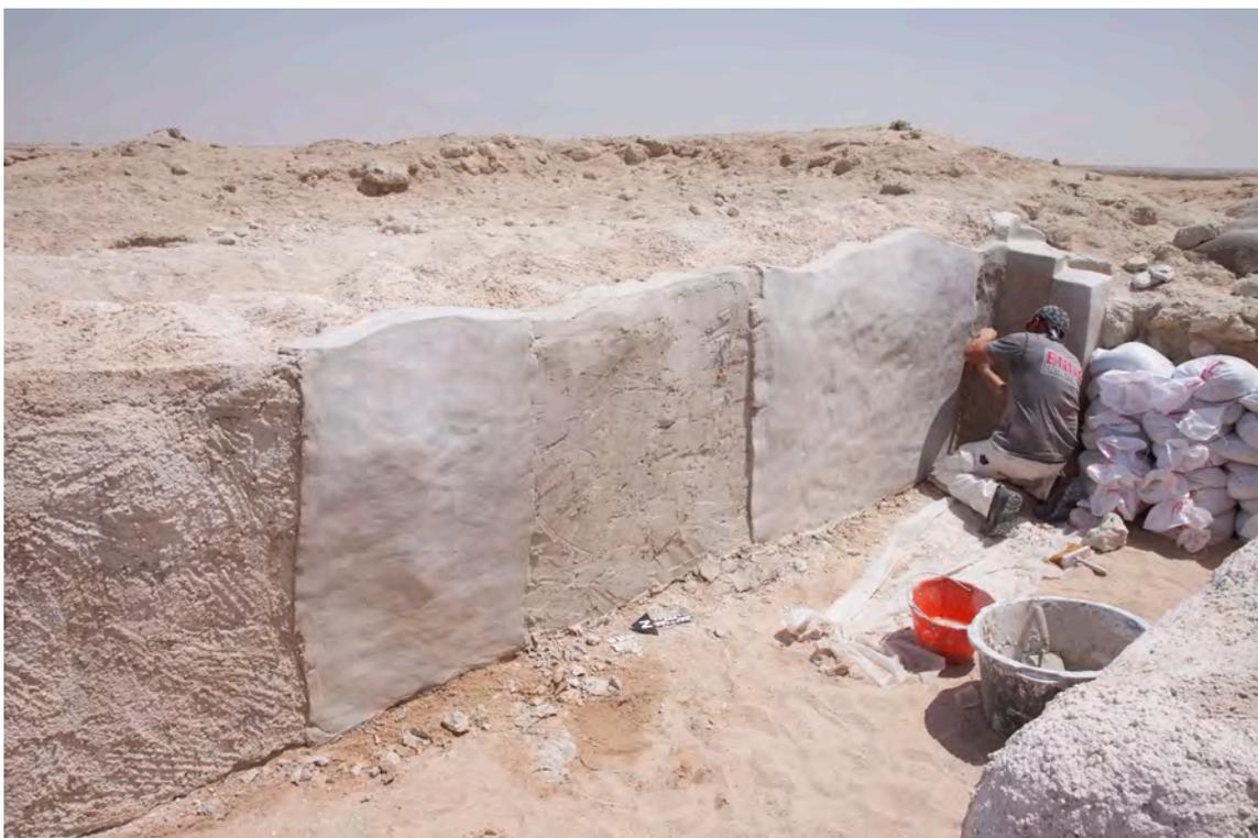
Figure 3.24: Gypsum plaster test fields in Space 3027. (DF-1131)
