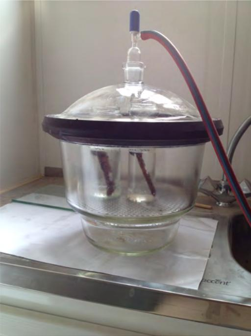
Figure 15.6: Two iron knives consolidated in a solution of 7 % Paraloid B72 and ethanol/acetone 3.2 under vacuum. (UG)
