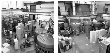
Figure 13: Neutron instrumentation at reactor SAPHIR 1983 with two-axis neutron diffractometers visible in the center of the pictures a) and b).
