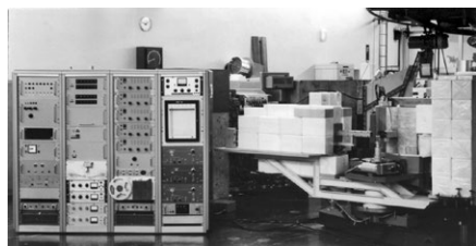
Figure 6: Powder neutron diffractometer with automatic data collection by means of paper tape input and output at DIORIT I.
