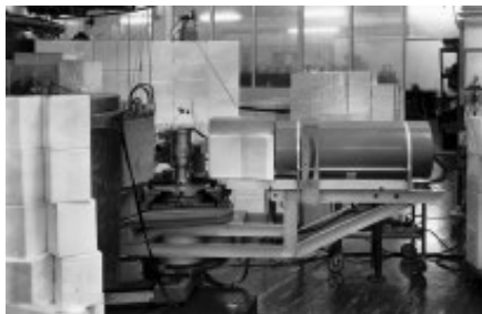
Figure 7: Optimized detector shielding at DIORIT I with optional counter tilting for single crystals.
