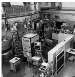
Figure 15: 7 mK refrigerator used 1988 on the two-axis neutron diffractometer P2AX@SAPHIR.
