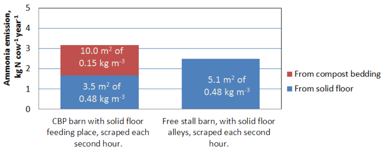
Figure 7. Estimated ammonia emission from a compost barn and from a free stall barn based on simple flux chamber measurements on CBP and on solid floor scraped each second hour.
