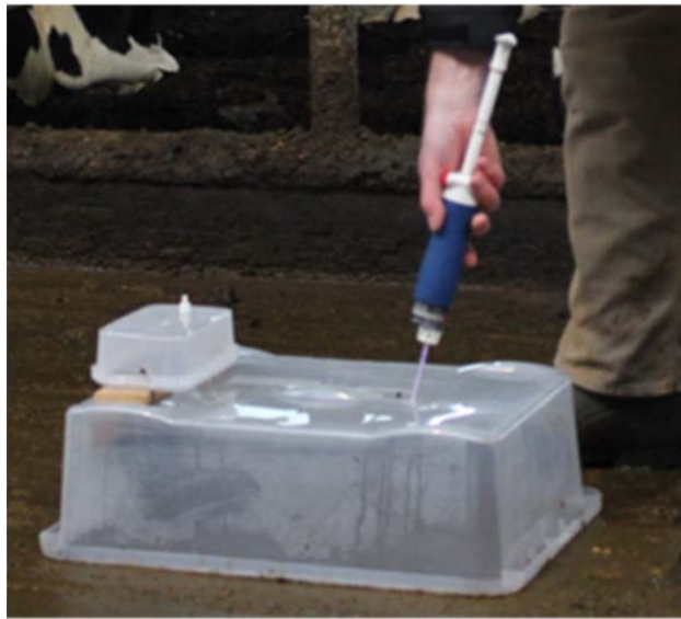
Figure 3. Simple flux chamber and a Kitigawa AP-20 sampling pump with 105SD detection tube for determination of ammonia emission.
