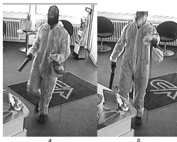
Fig. 5 After calibration, measurements may be done directly on the CCTV images
