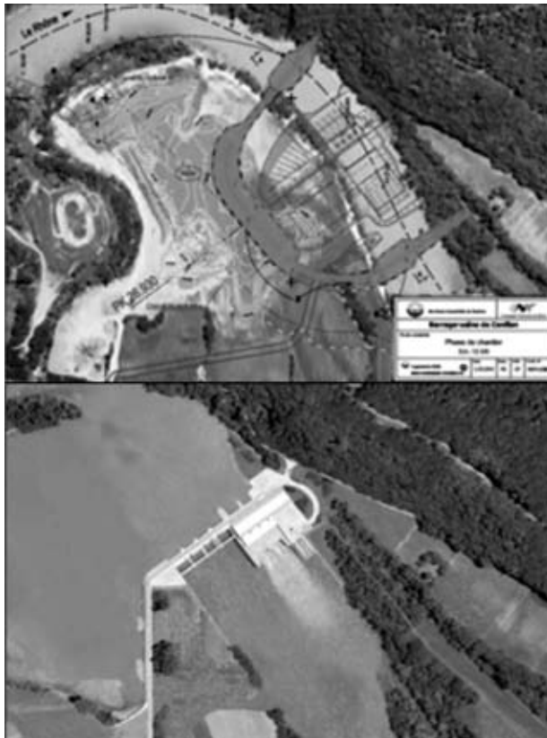
Fig. 1. Initial project plans superimposed on aerial view of the dam site at Conflan near Geneva (top). 3D simulation showing the impact of the water reservoir, dam and power plant (bottom). Courtesy of Laurent Niggeler, Service de la Mensuration Officielle, Département de l'Intérieur et de la Mobilité, Etat de Genève, 2011.
