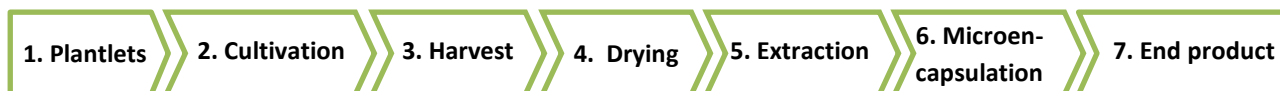
Figure 2. Production phases of a plant derived feed additive made ready to be mixed with a standard feed.
