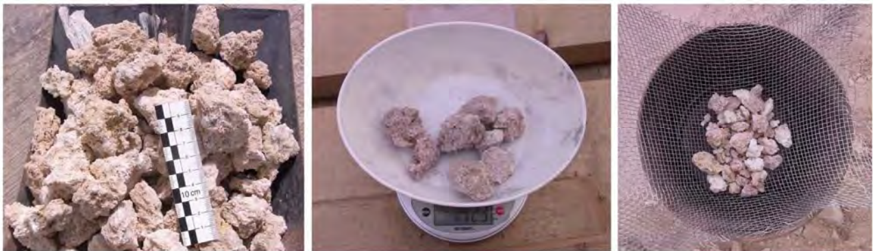
Figure 20: Selecting, weighing and sieving of raw material
