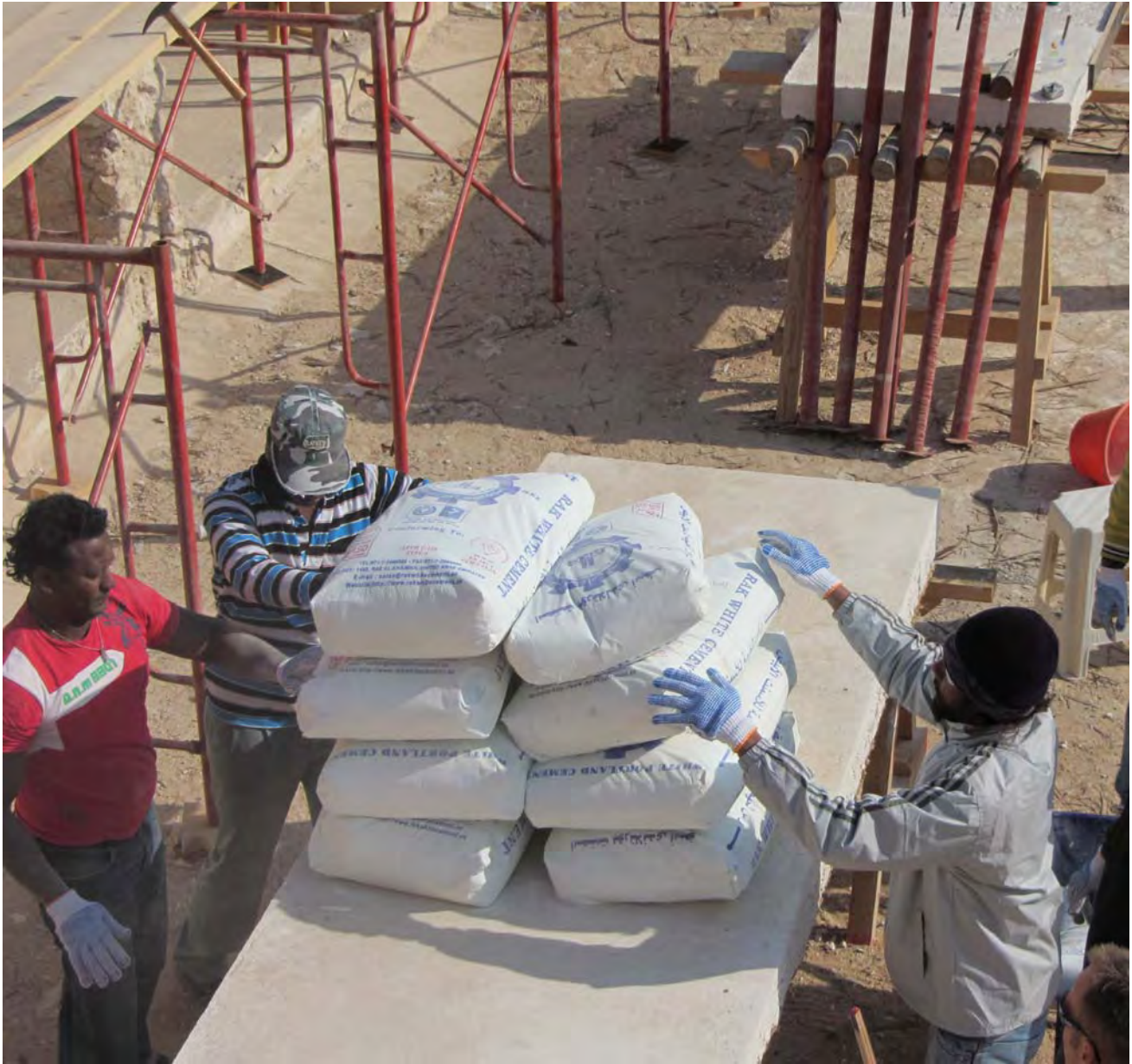
Figure 5: On-site bending tensile strength test
