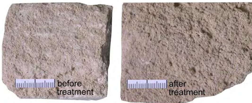
Figure 24: Gypsum plaster surface before (left) and after treatment with Xilan®. Note the slightly darker colour of the treated sample.
