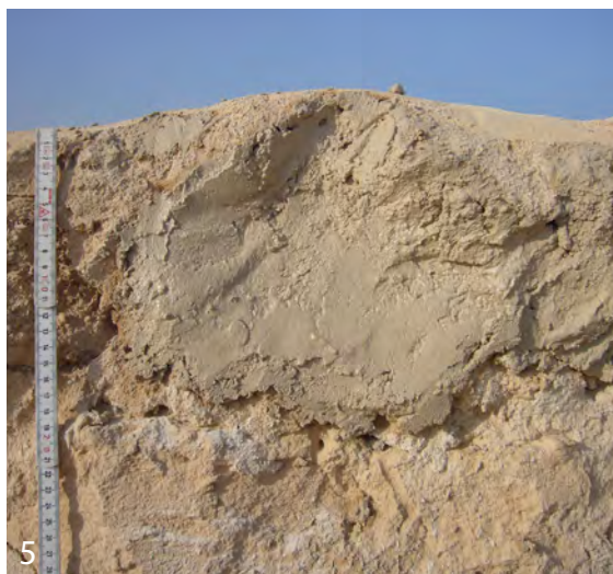
First mortar tests at Al Zubarah in November 2009: Soil mortar mix with the soil from the site. 1. Wall in QMA2 before test; 2. Close up on wall; 3. Mixing soil mortar; 4. Re-pointing of joints and fill of voids; 5. Fill hole to stone surface; 6. Same situation in December 2010.
