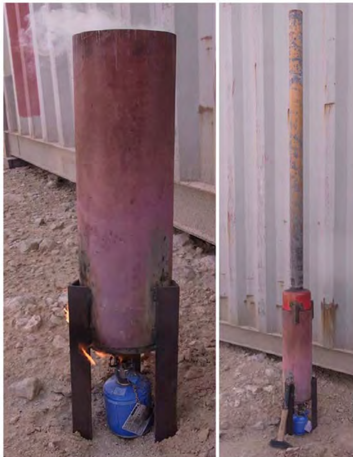
Figure 18: Large kiln with funnel mounted on top
