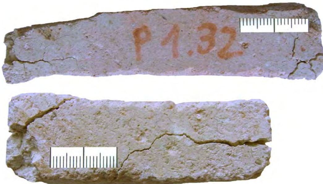
Figure 8: Sample “soil mortar” P 1.32 after 9 cycles in the water compatibility test
