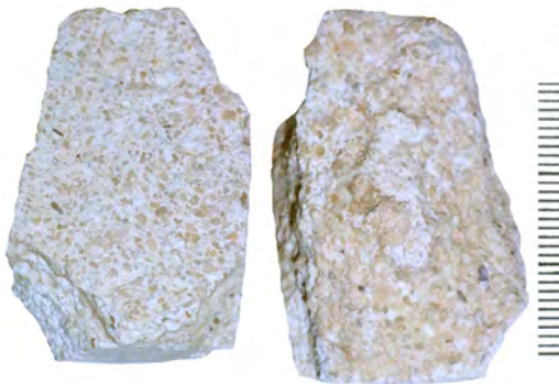
ZU 05 repair mortar from 1980
