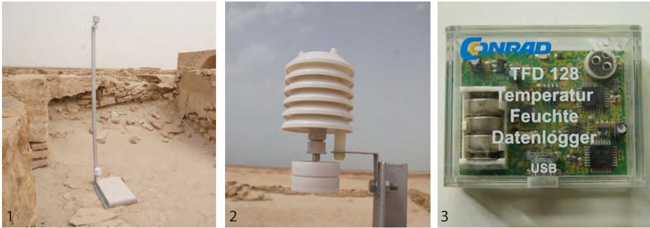
Fig.1, 2, 3: Temperature/humidity data loggers at QMA2 in Al Zubarah town (D1, D2) and HAB54506 at Al Zubarah Fort (indoor).
