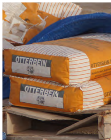
Natural Hydraulic Lime (NHL 5) produced by Otterbein
