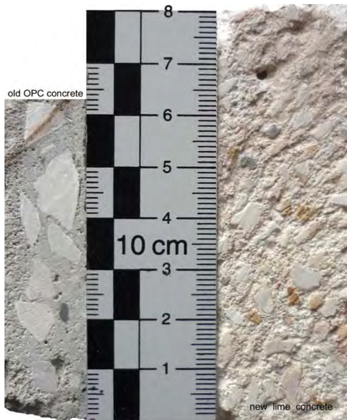
Figure 3: Old OPC (left side) and new lime concrete
