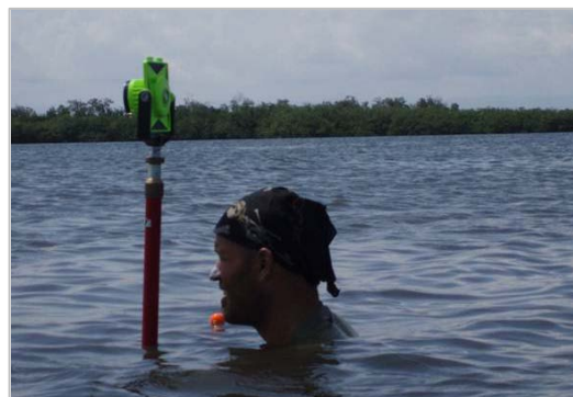
Figure 3. Student holding a prism pole on a wooden post for mapping (Photo by H. McKillop).
