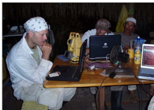
Figure 4. Total Station files are downloaded to a laptop at the Village Farm base camp and transferred to Excel files for attaching to the Project GIS, Underwater Maya (photo by H. McKillop).
