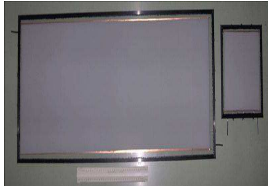
FIGURE 5.42. Prototypes of RPCs for performance studies. The larger chamber covers an area of 100 \times 30 \text{ cm}^2 .
