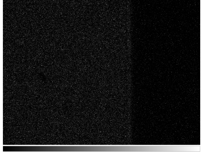
Fig. 4. Image captured by the EMCCD when it was exposed for 1 s with 10 flashes and a multiplier gain of 1000. The right third of the image was covered with black tape to provide a bias reference.
