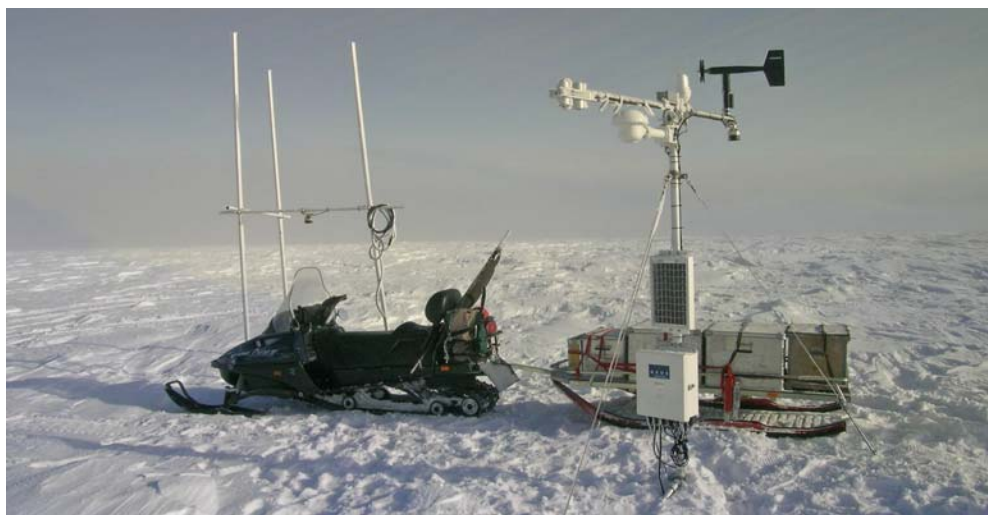
Figure 3.6 The AWS3 station near the Summit in May 2010 after minimal maintenance. Being in the accumulation area, the tripod is firmly frozen in the firn. Photo: Michele Citterio, GEUS.
