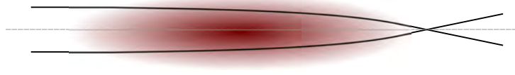
Figure 4.5: Illustration of lensing. The path of light rays through the atomic ensemble is bent and therefore diverges from a straight line - 1D model. The accumulated phase along the ray and therefore the resulting Faraday angle is altered.
