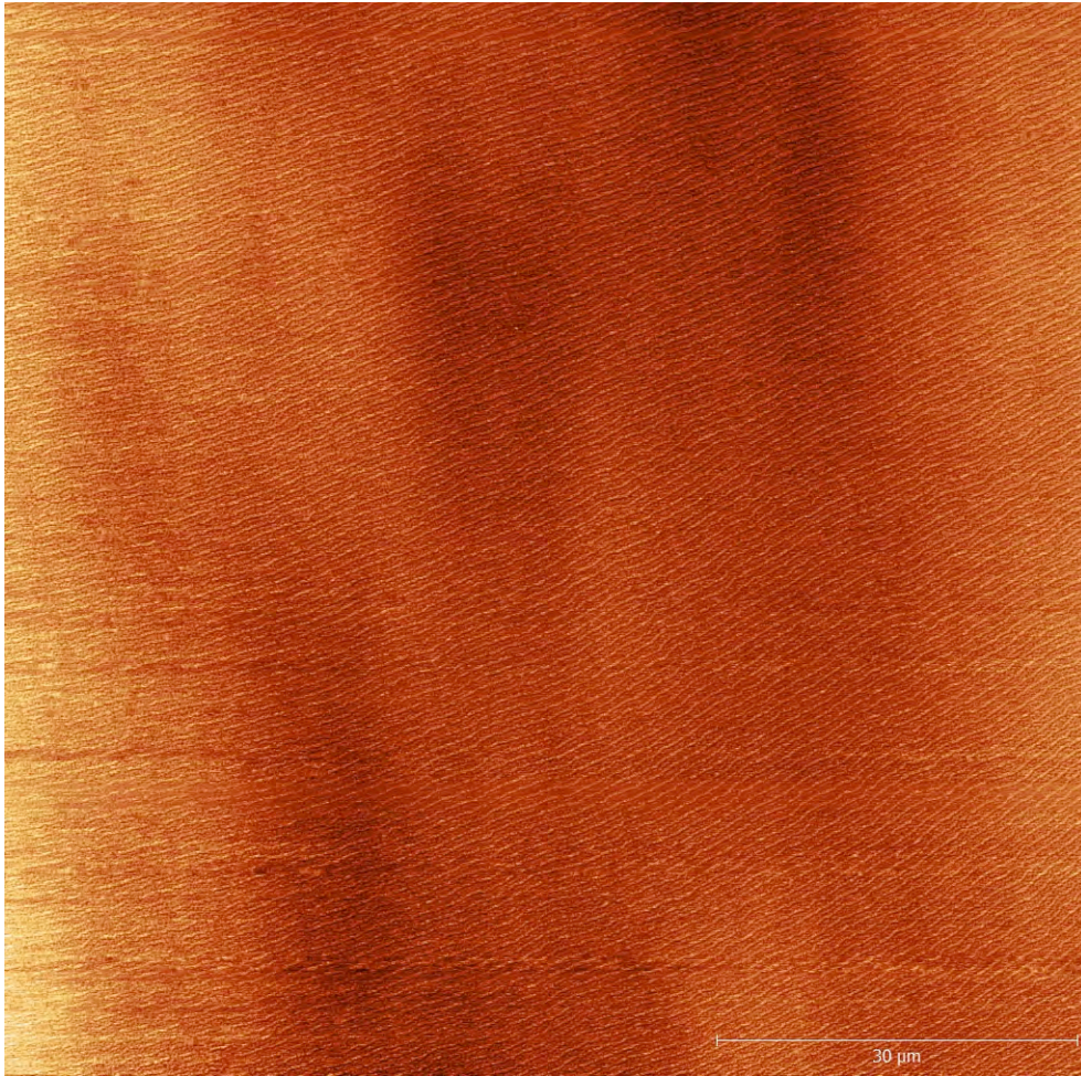
Figure 62: 90 \mu\text{m} by 90 \mu\text{m} AFM scan, showing that the stripe pattern covers huge areas with surprisingly few defects.
