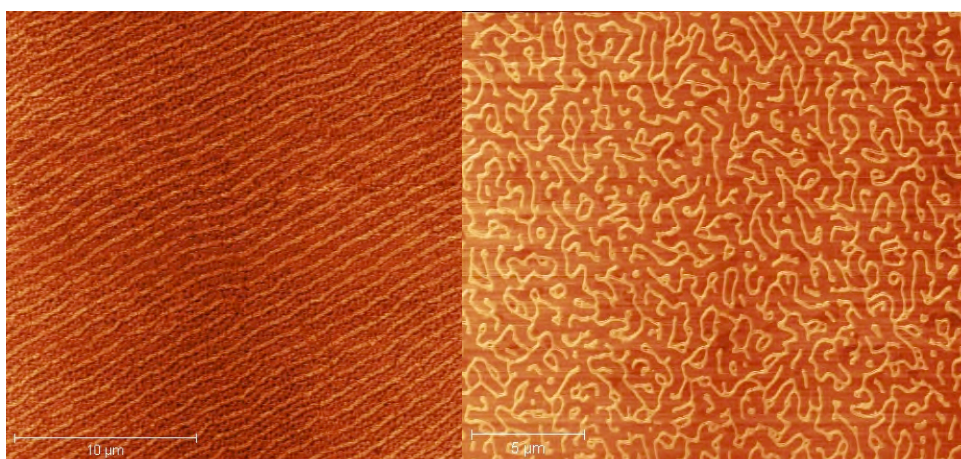
Figure 61: AFM pictures of DPPC on mica, deposited directly from a solution of 90% hexane / 10% ethanol. Left: The stripe pattern covering most of the surface of the mica. Right: Example of more complicated structure found in other rare places.
