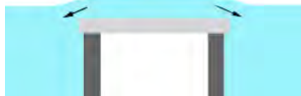
Figure 22. Visually assessing the level of water above the coverglass. Water drains slowly from the thin layer above the glass (arrows) this distorts the water surface. The thinner the layer and the faster the trough is drained the bigger the distortion. Experience with the specific trough and siphon allows a rather accurate and fast assessment. Dimensions of drawing are not to scale.
