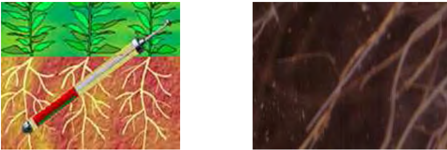
Schematic drawing of minirhizotron installed in soil (left hand side, © CID Inc.), and a subsample of a minirhizotron image (right hand side) showing roots growing outside the minirhizotron tube (sub sample image with area 1.5 x 3 cm).
