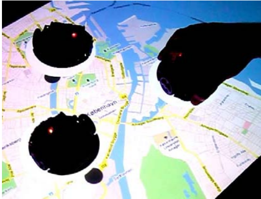
Figure 7. A map application using RoMo to allow panning and rotation of the map. Here, the user rotates the map by rotating a tangible.
