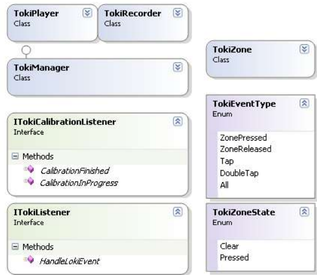
Figure 6: Main components of the Toki API.
