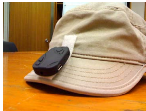
Fig. 1: The Ego-POV hat, mounted with key-fob camera
