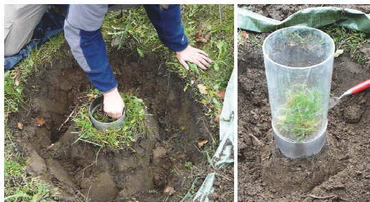
Fig. 15. Left: the stainless steel ring is placed on the soil monolith. Right: the soil column is gradually pushed downwards while making sure that no pebbles or roots get caught under the edge of the stainless steel ring.
