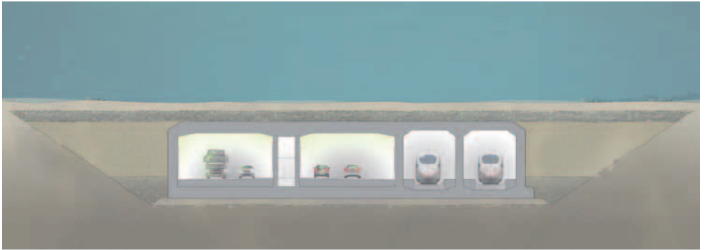
Figure 6. The special elements will ensure that ongoing operations and maintenance can be carried out without disrupting traffic. Beneath the road lanes and the rail track, there will be access to all technical rooms. Personnel, therefore, do not have to cross the traffic.
