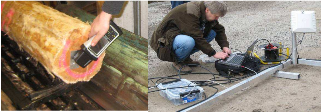
Fig. 3 Left: Hand-held reader operates only at very short distances Right: Experimental setup of antenna (top right) and computer for reading distances up to a few meters
