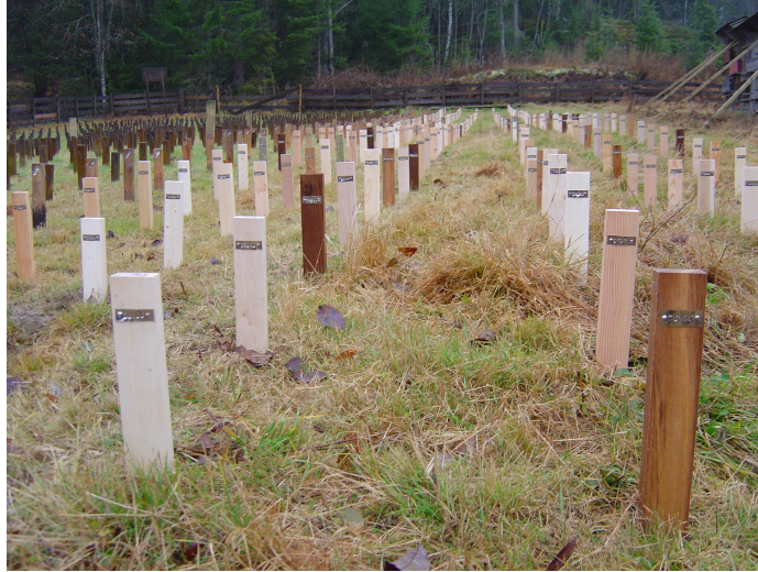
Fig. 1. EN 252 - field testing in ground contact (Sørkedalen, Norway).
