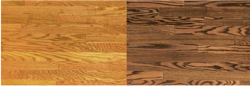
Fig. 4. Various dyes can be added to change the color of the impregnated wood.
