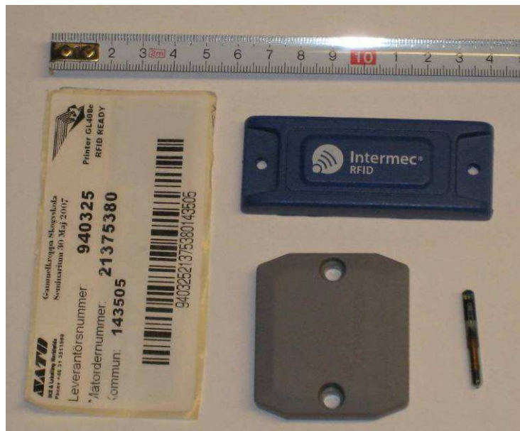
Fig. 2 Various tag types encapsulated in paper (left), glass (right, down) and plastic
