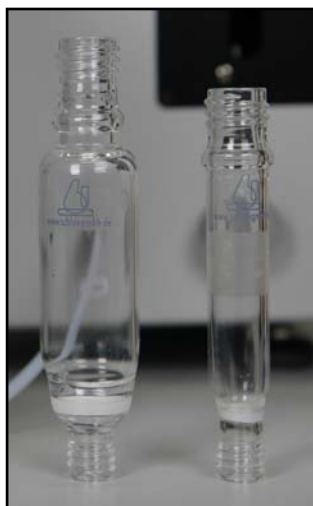
Figure S2. The custom-made, flow reactor vessels (10–20 mL and 2-5 mL) for the (SAMPS).
