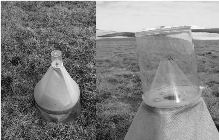
Fig. 5.5. Emergence trap placed in Sydkærene (left). Emerging arthropods are detained in the plastic cup by means of a simple lock (right).
