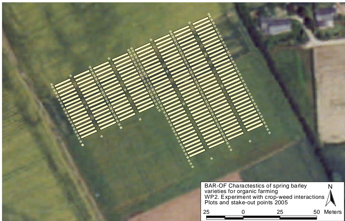
Fig. 1 Example of use of MarkGIS in planning and staking out the field trial in WP2 in 2005. Yellow squares show plots in the experiment from 2005 and the points show where sticks are placed helping the tractor driver having the right direction when establishing the field trial. The aerial photo used as background is taken in 1999.
