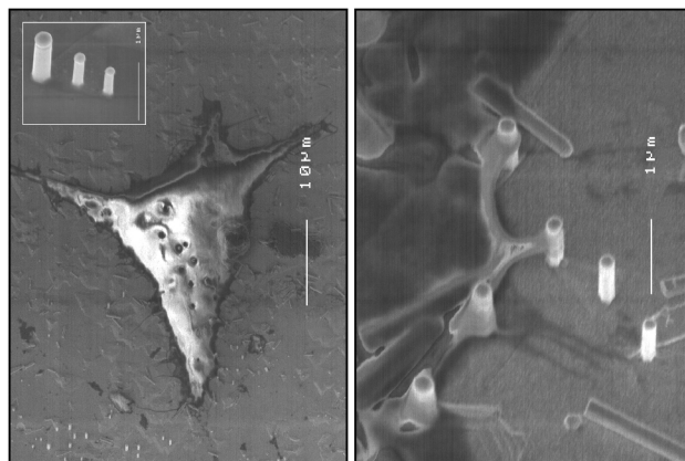
Fig. 2. (Left) Scanning electron micrograph of HEK293 cell cultured on an InAs NW array, scale bar 10 \mu\text{m} . Insert is a zoom on the NW array, scale bar 1 \mu\text{m} . (Right) InAs NWs embedded in HEK293 cell membrane, scale bar 1 \mu\text{m} .
