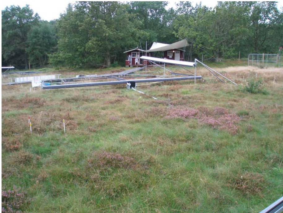
A: The CLIMAITE field site with temperate heath Deschampsia flexuosa and Calluna vulgaris vegetation. Left: ladder for vertical placement on the 7 m. diam. octagon (center) for safe-keeping the plots as non-disturbed. The right hand tall bar has the water exclusion curtain. The front low bar has the warming curtain.
