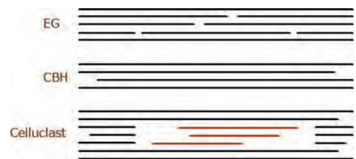
Fig. 7 Illustration of the enzyme action upon the structure of the cellulose matrix for endoglucanase (EG), cellobiohydrolase (CBH) and the cellulase mixture Celluclast 1.5 L
