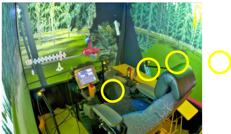
Figure 1. The four eye-tracking cameras mounted inside the simulator.
