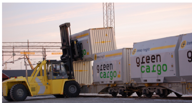
Offloading of 46 and 57 m 3 containers with a 42-ton forklift truck.
